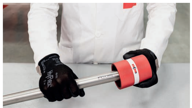
Figure 27 - Deburring the pipe
