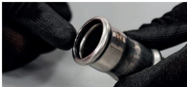
Figure 35 – Checking the sealing ring
