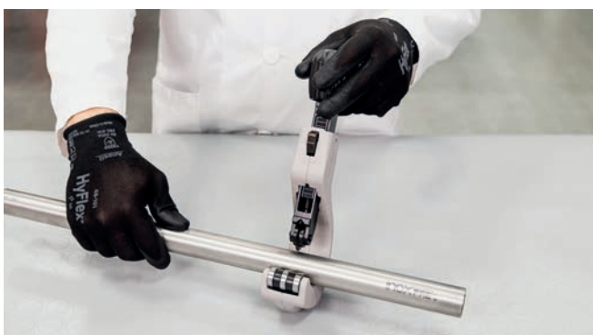
Figure 26 - Cutting the pipe to length
